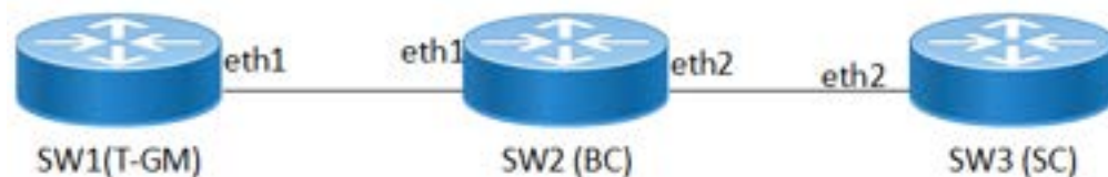
Figure 10. SMPTE PTP Configuration Toplogy
