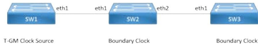
Figure 9. PTP IWF Profile Configuration
