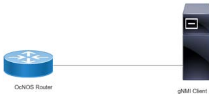
Figure 11. Dial-out Streaming Telemetry Topology
