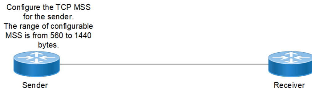
Figure 11. Configuring TCP MSS
