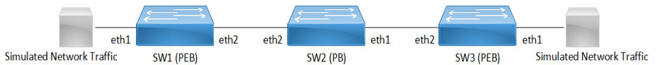
Figure 2-4: Single provider bridge configuration
