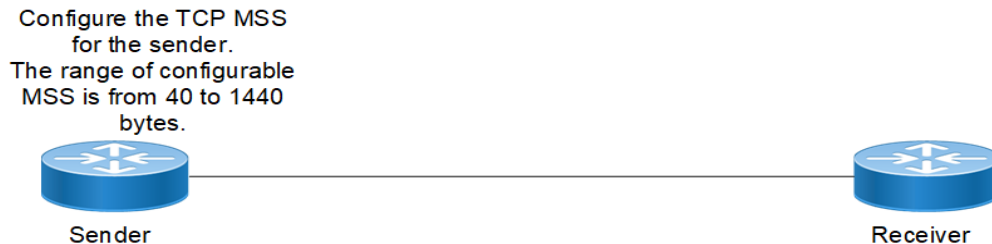
Figure 10-2: TCP MSS for BGP neighbor
