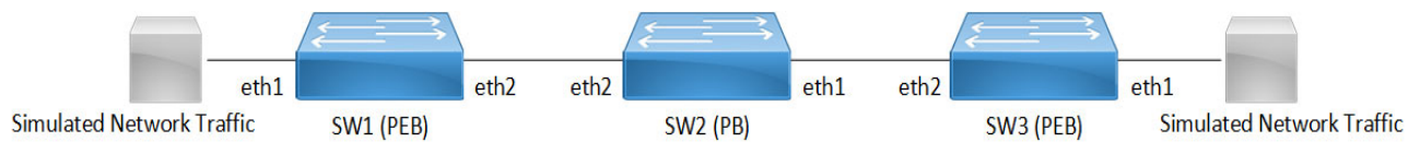
Figure 2-4: Single provider bridge configuration
