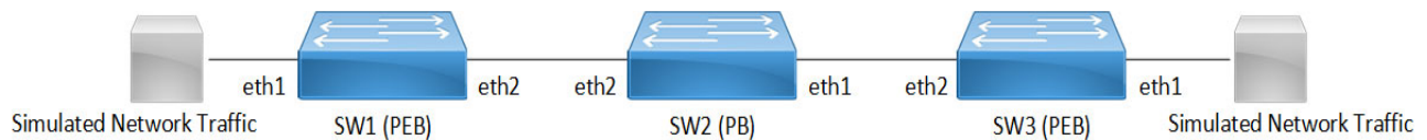
Figure 2-4: Single provider bridge configuration
