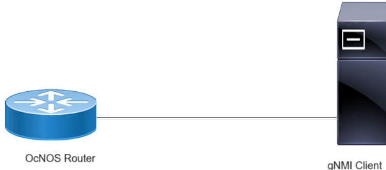
Figure 1-11: Dial-out Streaming Telemetry Topology
