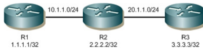
Figure 1-165: Basic Topology of Three Routers
