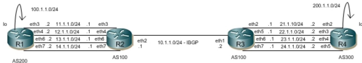
Figure 6-58: BGPv4 Additional Path Topology
