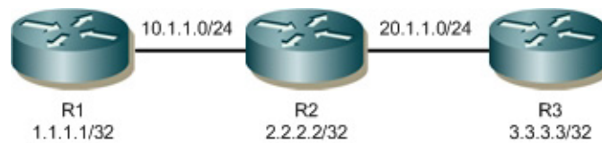
Figure 2-169: Basic Topology for BFD in BGP
