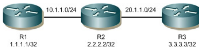
Figure 4-171: Basic Topology of Three Routers
