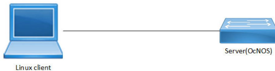
Figure 14-1: Netconf over TLS Topology
