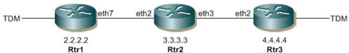
Figure 15-1: Three router topology for PW creation
