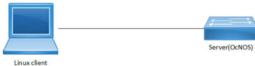
Figure 14-1: Netconf over TLS Topology
