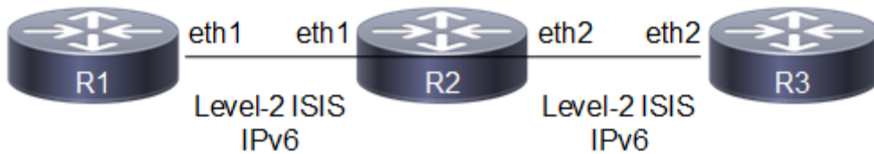
Figure 7-60: IS-ISv6 Passive Interface
