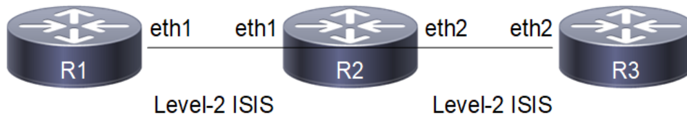
Figure 6-51: IS-IS Passive Interface
