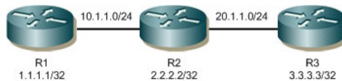
Figure 1-24: Basic Topology of Three Routers
