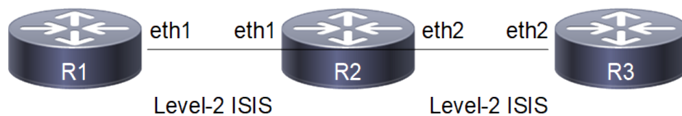
Figure 85. IS-IS Passive Interface
