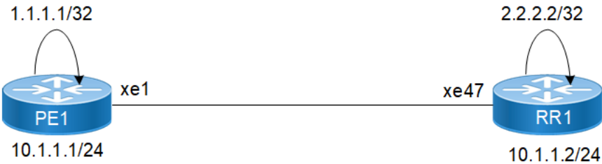
Figure 60. Device topology for BGP
