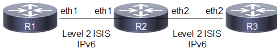
Figure 94. IS-ISv6 Passive Interface
