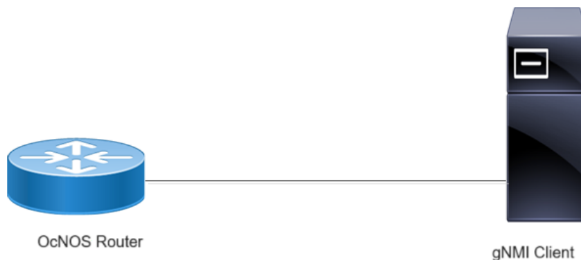
Figure 7. Dial-In Streaming Telemetry Topology
