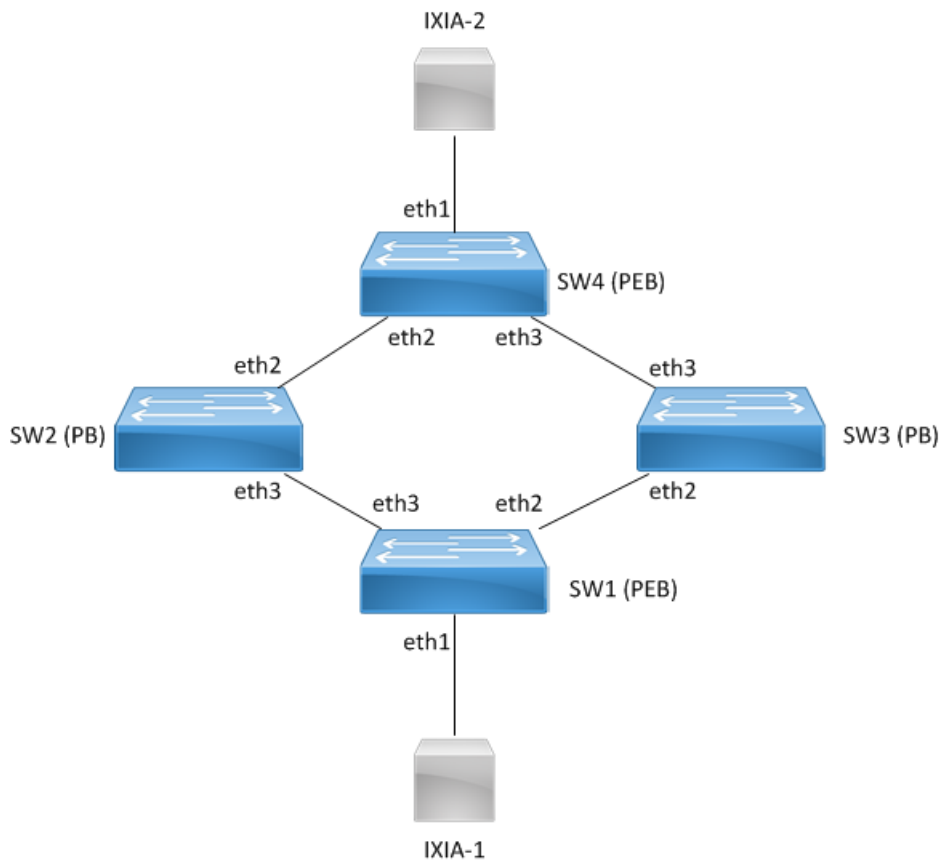
Figure 20-35: Two provider bridge configuration
