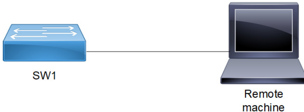
Figure 24-38: Syslog sample topology
