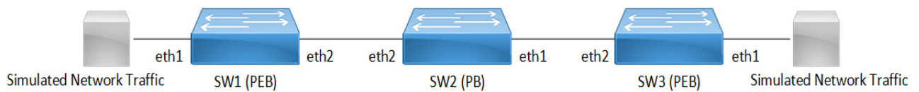
Figure 19-33: Single provider bridge configuration
